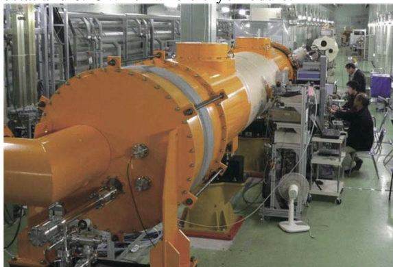
Figure 4 Four TESLA-shape cavity packages assembled in STF clean room (top). They were hung on the cryomodule cold-mass (bottom).
