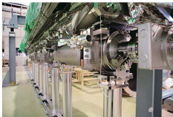
Figure 4 Four TESLA-shape cavity packages assembled in STF clean room (top). They were hung on the cryomodule cold-mass (bottom).
