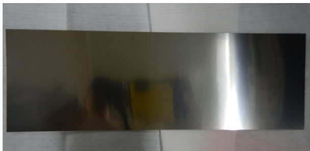
Figure 3: 20 \mu\text{m} \times 100 \text{mm} \times 300 \text{mm} stainless steel foil.
