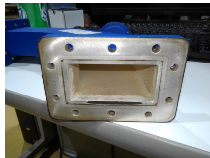
Figure 5: Photograph of the damage on the waveguide due to RF induced breakdown.
