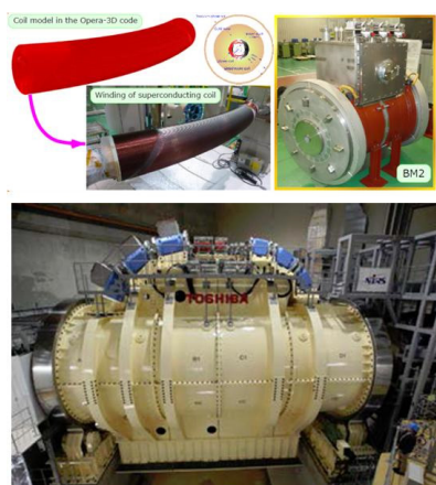
Figure 2: Rotational gantry for heavy ion radiotherapy at NIRS and the superconducting magnets.
