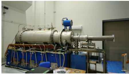
Figure 2: Repetitive pulsed-power generator “ETIGO-IV”.
