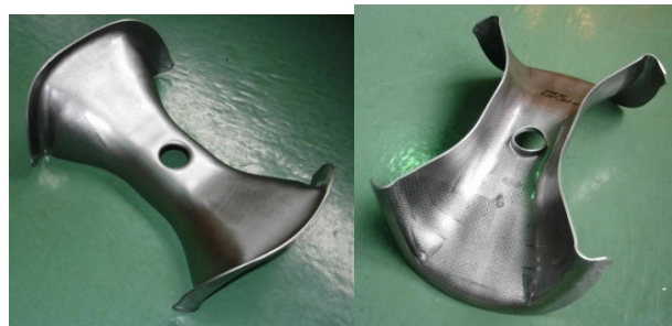
Figure 1: Press formed shape after burring with niobium sheet of 2.5 mm thick.
