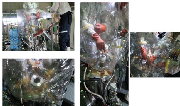
Figure 8: Refrigerator replacement work.
