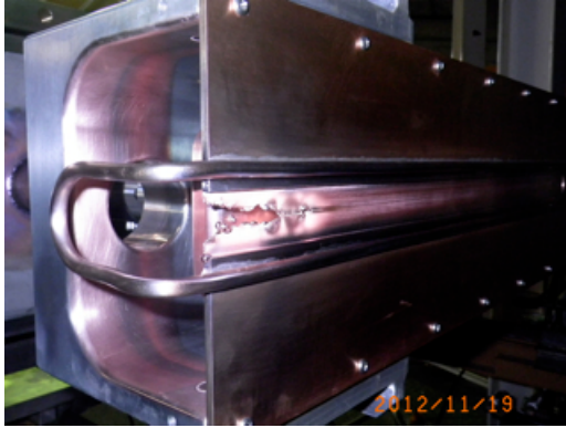
Figure 9: Melted septum of RRC-EDC caused by the large beam loss of 1.5 \text{ kW} .
