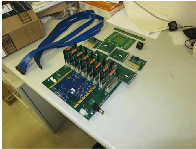
Figure 9.45: 64-channel motherboard for development, with digitizer daughter cards.
