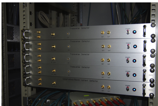
Figure 9.22: Picture of the transverse and longitudinal detectors installed in a rack.
