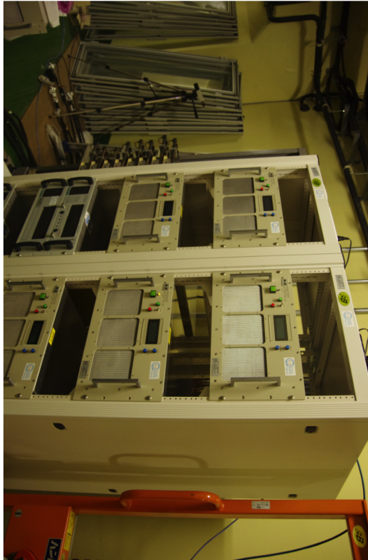
Figure 9.25: Longitudinal feedback amplifiers.
