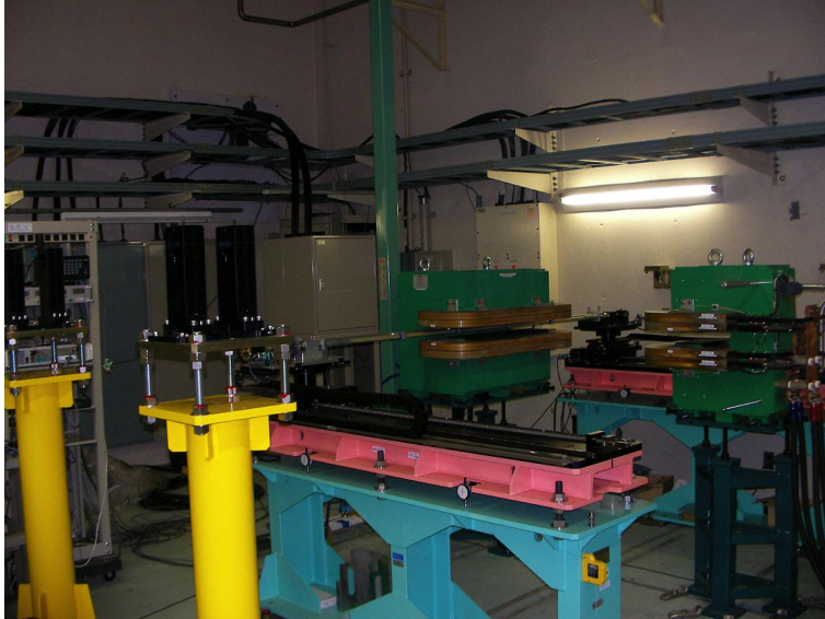
(b) Harmonic coil system for the multipole measurement.
