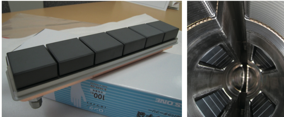
Figure 12.46: The left photograph shows a unit of the HOM-absorbing structure; six SiC ceramic tiles are brazed on a water-cooled copper plate, and a stainless-steel frame is also brazed on the perimeter of such plate for TIG welding. The right photograph shows an inside of a GBP with four rectangular openings, in each of which such unit is fitted, and this GBP is hermetically sealed by TIG welding.
