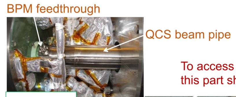
To access QCS pipes & BPMs, this part should be disassembled.
