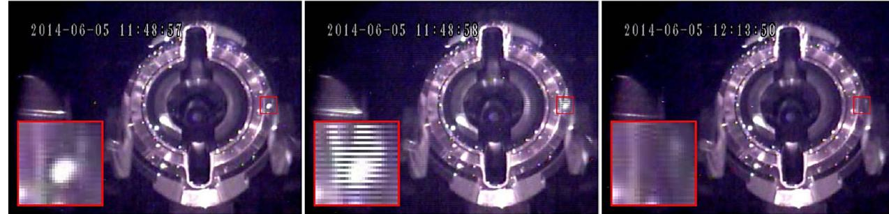
(a) 1 frame (1/30 s) before this cavity breakdown.
