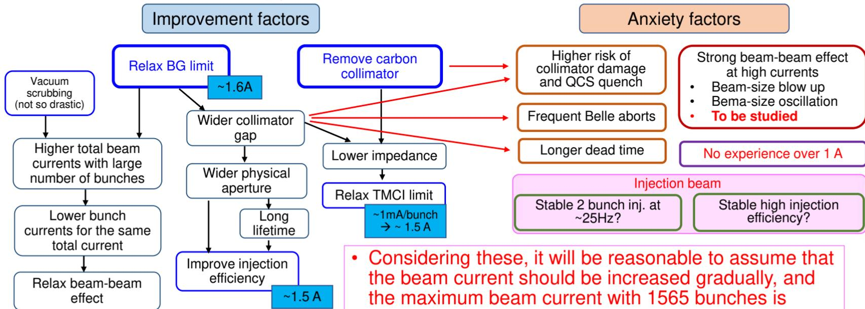
Considering these, it will be reasonable to assume that the beam current should be increased gradually, and the maximum beam current with 1565 bunches is **1.1~1.2 A (0.7~0.8 mA/bunch)** for 2021a and b runs.
