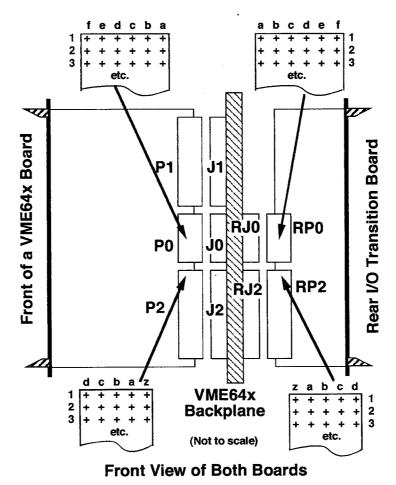
**Note:** Connectors RJ1 and RP1 are not normally used and therefore are not shown. If these two connectors are used, care should be taken when connecting to the VME64x bused signals and to the power pins.
